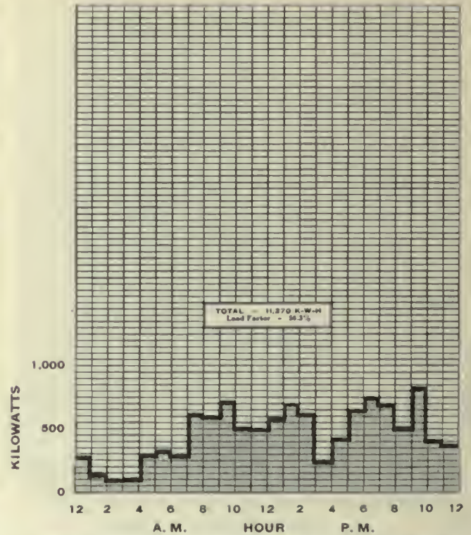
FIG. 602. ENERGY CHART. Kilowatt-Hours at the Pantograph for the Average October Day for 11,000-Volt A. C. Operation, Passenger Transfer Service.
